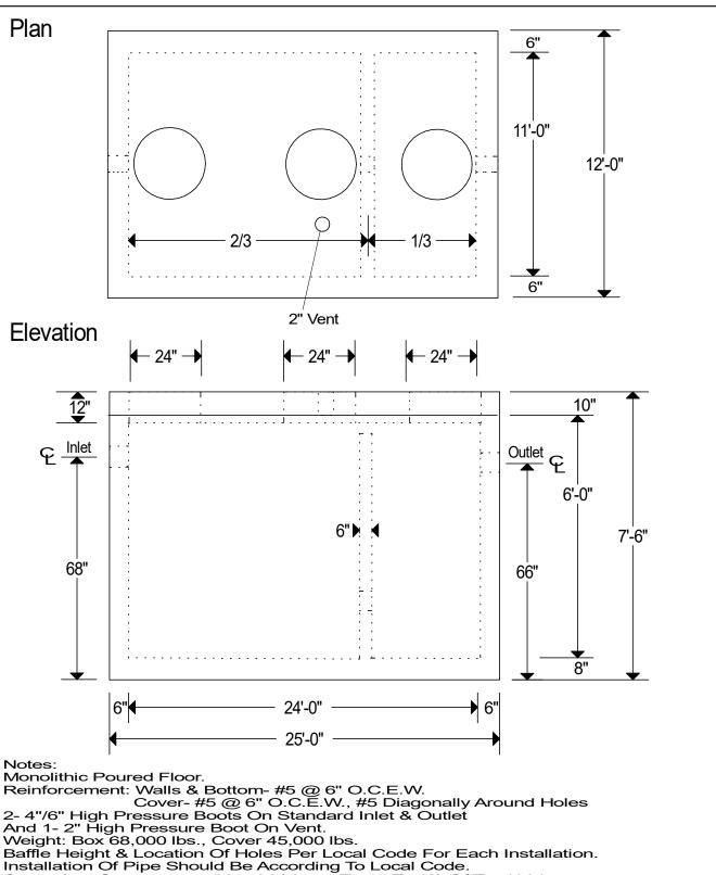
Secondary Compartment Has A Volume Equal To 1/3 Of Total Volume. 5,000 P.S.I. Minimum Strength Concrete.
